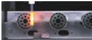
Correct positioning of the ignitor over the burner is essential for proper ignition.
